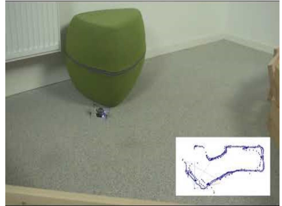
Example of CrazyFlie Multi-Ranger Deck point cloud
